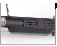
Locate the Ruger mini top cover plate with new top picatinny rail attached.
