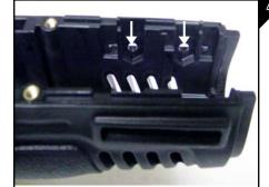
To install the side rails locate the existing pockets on the inside of the stock and insert the (2) 6-32 hex nuts into the pocket as seen in Figure 4.
