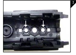
Align the side rail into place and holding a finger over the hex nut, use a phillips head screwdriver to fasten the (2) 6-32 x 3/8" machine screws to the picatinny rail as seen in Figure 5. Repeat for the opposite side picatinny rail installation.
