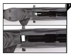
After installing the trigger assembly make sure to function check your Mini-30 to insure that the bolt is cycling properly. If your bolt sticks during any portion of the cycle you may have to add a 3/32 x 5/8" shim between the trigger assembly and stock as seen in Figure.
