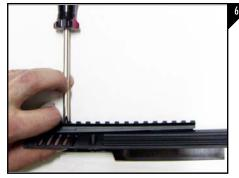
To install the top picatinny rail, insert the (4) 6-32 hex nuts into the pockets on the reverse side of the top cover. Holding the hex nut in place and using a phillips head screwdriver fasten the (4) 6-32 x 5/16" screws to secure the top cover as seen in Figure 6. To install the Stainless Steel Insert please refer to Figure 1.
