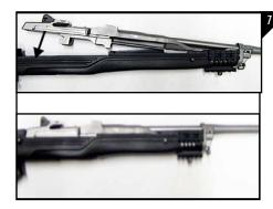
To install the barreled action, align the barrel to the front of the stock and bring the rear down towards the rear of the stock and firmly secure the barrel in place as seen in Figure 7.
