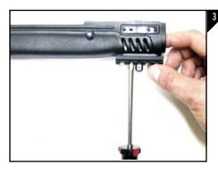
Align the bottom picatinny rail into place and holding a finger over the hex nut, use a phillips head screwdriver to fasten the (2) 6-32 x 3/8" Machine screws and bottom picatinny rail into place as seen in Figure 3.
