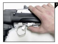
Align the trigger assembly and insert back into place. Lock the trigger assembly by firmly pushing the trigger guard up and into the locked position as seen in Figure 8.
