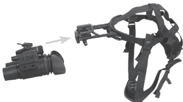
FIGURE 3-10. ATTACHING ATN PS15 TO PVS HEAD MOUNT
