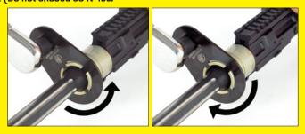
9 Install the gas block & gas tube.
