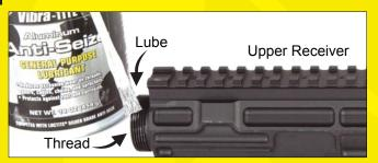
Test fit the barrel nut on the upper receiver by hand tightening it on, then remove.
