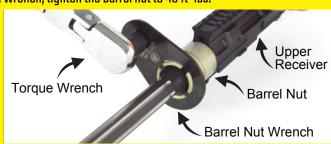
Loosen the barrel nut one-half turn and re-torque to 45 ft-lbs. (Do not exceed 50 ft-lbs.
