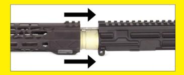
Insert the rail retention clamp into the the RIGIDRAIL... and tighten the hex bolts to 30 in-lbs. Alternate torque between each screw until they both stop rotating when torque is applied.
