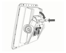
5 Press the button on the lever, and push the lever down until the device clicks in place.
