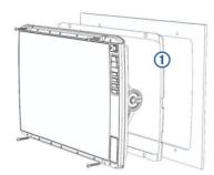
**12** Connect all necessary cables (*Connector View*, page 4), and spin the locking rings clockwise to secure the cables to the cradle before placing it into the cutout.
