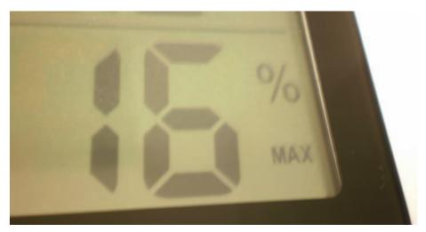
Press the MAX key to view the maximum values recorded since the last time they were cleared. **Note:** Max must be displayed when the clear button is pushed to clear.
