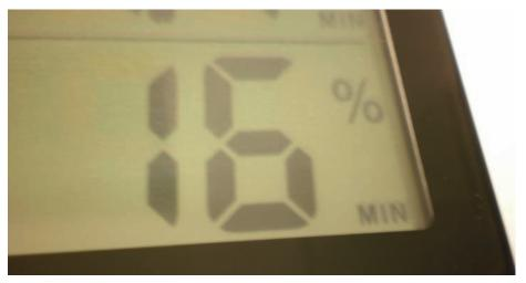
Press the MIN key to view the minimum values recorded since the last time they were cleared. **Note:** Min must be displayed when the clear button is pushed to clear.
