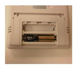
The hygrometer uses one (1) AAA battery. If there is an extra battery slot it is for storing a spare battery only. The minus (-) end of the battery goes against the spring, the positive (+) end goes against the contact with the dimple.
