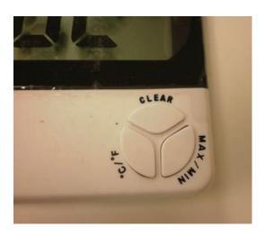
Use the C°/F° button to select Fahrenheit or Centigrade scale. Use the CLEAR button to clear minimum or maximum values that have been stored in memory.
