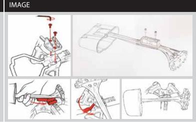
For side-mount bracket, attach side-mount bracket to picatinny rail on bottom of crossbow stock using included hardware. Slide quiver into side-mount bracket. Close locking lever.
