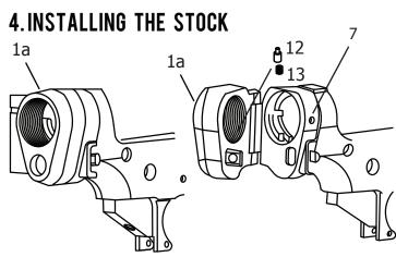
With the folding stock adapter tightly installed on the receiver, using a 3/32 Allen Wrench, tighten Flange Set Screw (7) to secure the Threaded Flange. Make snug but do not over tighten.
