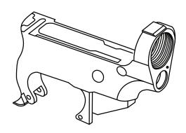
Ensure the weapon is unloaded with the safety engaged! Remove the stock from the rifle, remove the buffer and action spring from the buffer tube, and then remove the buffer tube (receiver extension) from the receiver. When removing the stock and tube from the receiver. For detailed information on removing the stock assembly from the receiver, refer to the firearms manual.
