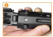
Test for handguard alignment by carefully sliding the handguard over the barrel nut ensuring that you can see the barrel nut's channel centered within the hole cut out in the handguard.
