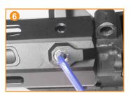
Carefully slide the handguard back on until it meets the receiver and tighten the two handguard screws. Recommended torque value is 15 in-lb. Do not overtighten.
