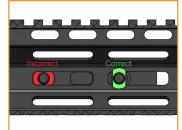
If the T-Nuts are spaced with too much gap they will rotate freely when trying to tighten. Alternately, if the T-Nuts are not spaced with enough gap they will not rotate at all. Observe the T-Nut during the installation process to be certain that they have rotated to their correct position as shown.
