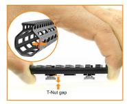
In order to properly secure a rail section or other M-LOK® accessory on your rail system, the T-Nut gap must be slightly larger than the rail thickness. Either measure the rail thickness or use the edge of the rail as a gauge.
