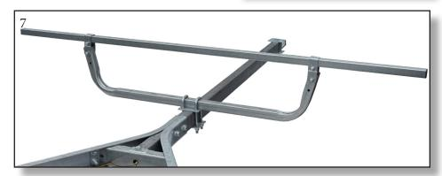
**Step 8**. Install the D-Rings to the ends of the load bars. Slide a nylon lock nut into the open end of the load bar and align with the hole. INSERT and hand tighten the bolt.
