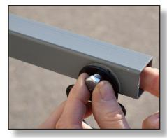
**Step 9**. To secure, Slip a screwdriver under the nylon nut to hold it in place as you fully tighten the bolt with a 9/16 socket wrench. Complete the cross bar with the new end caps.
