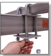
**Step 5**. Slip the new load bar brackets over the new load bar (as shown) and loosely install the two small bolts / nuts through each bracket trapping the load bar inside the brackets. See Figure 5
