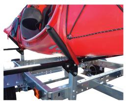
7). Bring the strap back up and through the cam buckle. Pull down to tighten. Repeat strapping for second kayak
