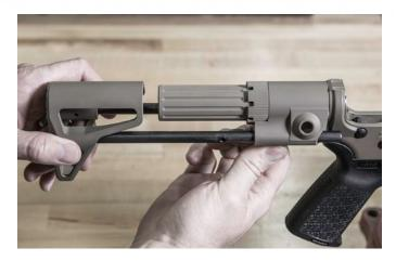
**STEP 6:** Squeeze the adjustment lever and take down lever together and insert guide rods of stock into the housing. Once past the first stop, you will only need the larger adjustment lever to adjust length of pull.
