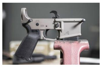
**STEP 1:** Secure your lower receiver into a vise block. Remove your existing stock if one is installed. NOTE: You will not need the stock end plate when using the PDW Stock.
