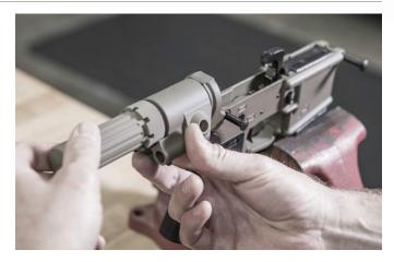
**STEP 2:** Ensure the receiver extension is inserted into the stock housing and your rear takedown pin detent and spring are in place. Begin to screw the receiver extension into your receiver. Do not completely tighten.
