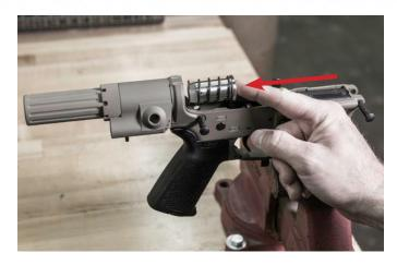
**STEP 5:** Insert proprietary buffer assembly, either the Maxim Buffer & Spring, or exclusive JP Silent Captured Spring
