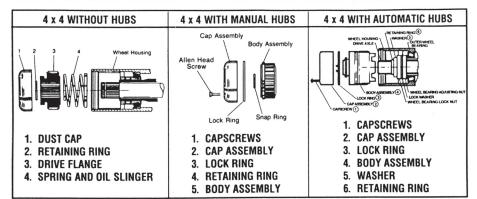
Notice: Hub leaves manufacturer with proper amount of grease. Verify lock nut tightened to manufacturer's specified recommended torque. Loose wheel bearing adjustment will result in damage to hubs.
