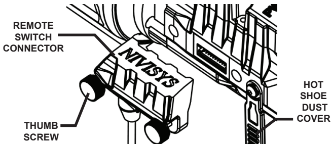
Figure 2-13 Remote Switch Installation
