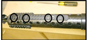
2. Remove the clamp bar from the rail and then roll the rail onto the receiver and the forearm rail. Then line up the 2 lugs on the forearm rail with the 2 chamfered holes on the rail.
