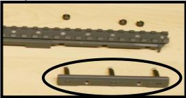
3. Once the alignment is good install the 2 flat head screws that come with the rail. Snug
