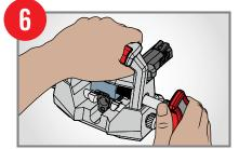
Turn Easy Torque Handle™ and push through dovetail slot.
