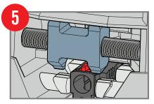
Confirm alignment with Press Block and sight.
