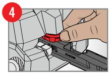
Snugly tighten vertical stabilizer to hold pistol
