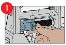
Select applicable Press Block face and center over pistol slide in tool cradle.
