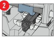
Align clamp guidelines with center of dovetail and secure slide in cradle.
