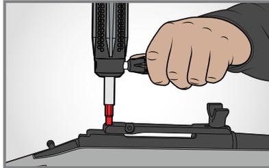
A properly torqued base is critical to mounting a scope for accuracy whether on a rail system or receiver. Adhering to the manufacturer's torque specifications assures that the scope will be securely mounted to the gun.
