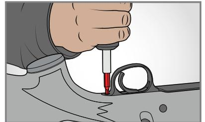
Easily tighten fasteners to the manufacturer's recommendation when adding accessories or changing/upgrading the stock. Correctly torquing the screws that attach the stock to a barrel assures you of safe and accurate operation.
