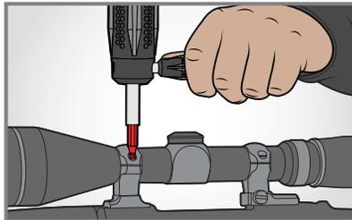
Overtightening rings is the number one cause of scope damage/failure. Most scope rings are steel, scope tubes are aluminum. Always follow the manufacturer's precise recommendation for torque and never crush a scope tube again.
