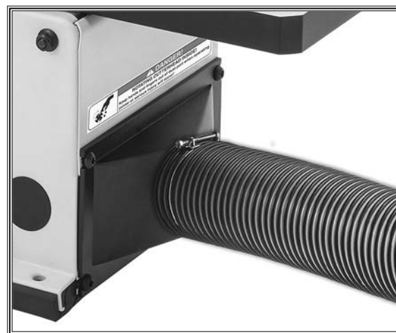
Figure 16. Dust port connected to dust collection system.
