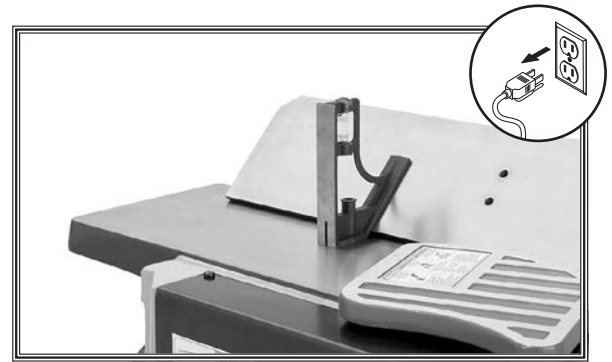
Figure 41. Example of checking 45° outward fence angle.
