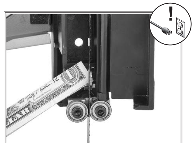
Figure 26. Dollar bill folded twice to make a quick 0.016" gauge.
