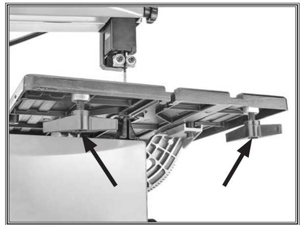
Figure 14. M6-1 x 16 fence rail knobs installed.
