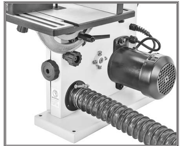
Figure 22. 2" dust host attached to dust port.
