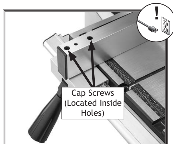
Figure 33. Location of the fence adjustment cap screws.
