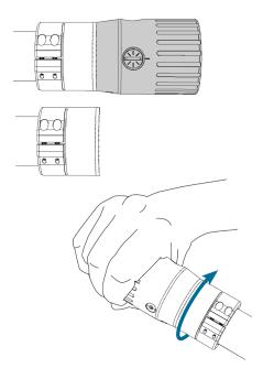
To reinstall the lens, align it to the mount section and carefully thread the lens on by turning it clockwise onto the mount section. Fully thread the lens onto the mount section until the alignment markers are realigned as shown.
