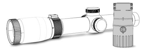
ongratulations on your purchase! The TRYBE™ OPTICS Enhancer doubles the power of most 34mm, 30mm, or 1" scopes by attaching to the end of that size scope tube. Simply connect to your existing sighted-in riflescope and zero the Enhancer. Then just remove or replace the lens to double your magnification with no further adjustment required.
