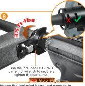
Attach the included barrel nut wrench to a torque wrench and seat the teeth of the barrel nut wrench into the second slot of the barrel nut (closest to the receiver). Securely tighten the barrel nut by turning clockwise. Recommended torque value is 35 ft-lbs.
