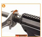
To remove the stock handguard barrel nut, use a 1-3/8" wench or equipped breaker bar to mate with the flats found on the barrel nut and turn counterclockwise, 35-50 ft-lbs of torque will need to be applied for removal.
