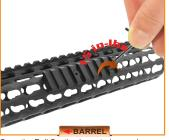
Once the Rail Section is seated properly, use the included 3/32" Hex Wrench to hand-tighten the screws on top of the Picatinny Rail Section to lock it securely to the Keymod Compatible Handguard. Do not over-torque. Apply (15 in-lb) torque to secure screws
