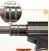
Make sure none of the locking ring's 6 threaded screw holes are blocked by the barrel nut. If they are blocked, refer back to step 7 to install a spacer(s) or tighten the barrel nut further, if the blockage is only minor.
