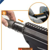
Slide the included locking ring into the barrel nut, making sure the alignment slot on the locking ring is vertical and facing upward.
