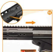
Carefully slide the handguard over the barrel nut/locking ring assembly. Make sure the handguard sits flush up against the receiver with its top rail aligned with that of the receiver top rail. There should be little to no gap between the two. If you lose the vertical alignment of the locking ring, use the included T20 Torx wrench to fix the alignment and correctly position the locking ring's threaded screw holes with that of the holes found on the handguard.
