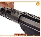
Secure the rifle in a padded vice or by using a correctly sized magazine well vice block. Make sure the rifle is secured in such a fashion as to allow access for removal of the stock handguard
