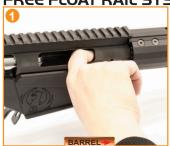
While following all basic rules of firearm safety, first ensure the firearm is unloaded by removing the magazine and pulling the bolt to the rear to physically and visually check the chamber to be empty.
