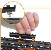
Place the rail with the Keymod Nuts onto the desired slots of the handguard, inserting the nuts through the larger opening of the Keymod Slots with the protruding feet of the nuts pointing toward the muzzle of the firearm.
