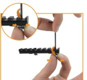
Hold the Keymod Nut in place and loosen the screw by turning it counter-clockwise with the included 3/32" Hex Wrench. Do not fully detach the Keymod Screw from the Keymod
