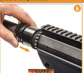
With the stock handguard barrel nut now removed, slide the included barrel nut onto the barrel and thread it clockwise onto the receiver threads until hand tightened.
