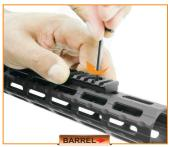
Insert the supplied Hex Key into the rail section screws and rotate them clockwise. Apply a maximum of 30 in-lb.
