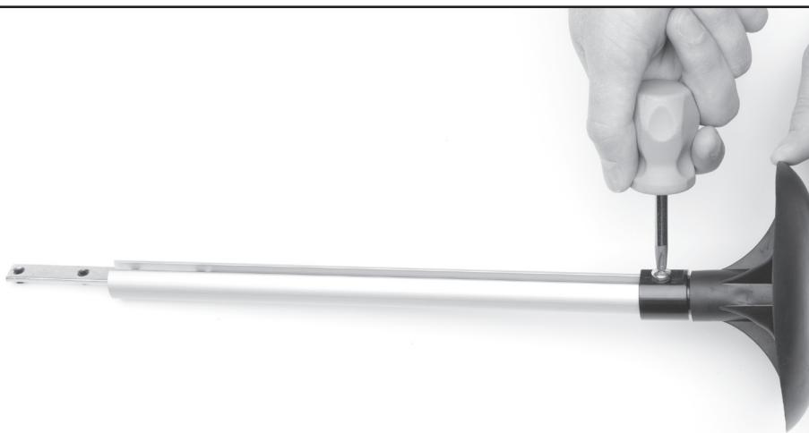
Identify the side of the part that has the foot attached to the aluminum bar. Slightly loosen the Phillips Screw (roughly 1 full turn) so the foot will slide off the end of the aluminum bar.
