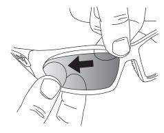
Replace the lens into the frame by positioning the temple edge of the lens into the frame. Be certain the edge of the lens is centered into lip of the frame.
