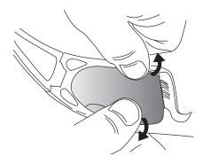
Place hands as pictured above with thumbs on the inside of the frame. Grasp the upper and lower portion of the frame and pull apart. When you feel the frame give, apply pressure with your thumbs on the lens.
