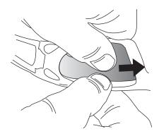
Push the lens out of the frame and slide lens toward nose bridge.
