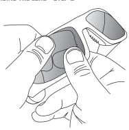
Press the edge of the lens into the frame as pictured above, "walking" the lens into the frame and finishing at the nose bridge. Double check to be certain the lens is seated evenly into the frame.
