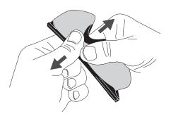
Position one hand to grasp the frame at the center of the brow bar, the other hand directly opposite at the nose piece lens junction, as pictured. Simply pull apart.
