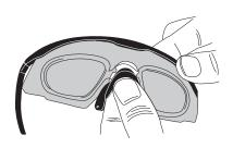
Align the groove of the nose piece into the primary lens.
