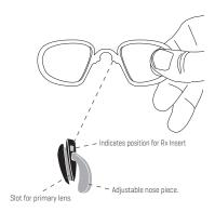
The prescription insert is held in place by aligning the buds on the Rx Insert into the notches on the nose piece.
