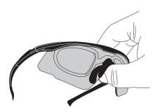
Position hand as pictured above and squeeze into lens until the nose piece completely seats.
